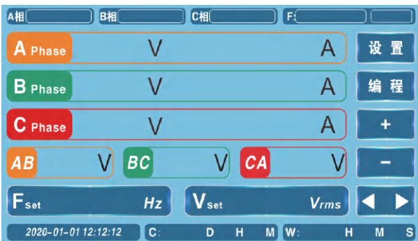
Main interface of three-phase power supply
