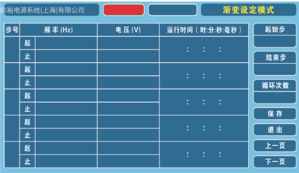
Gradient Setting page can set the required voltage and frequency, Run time, initial step, end step
