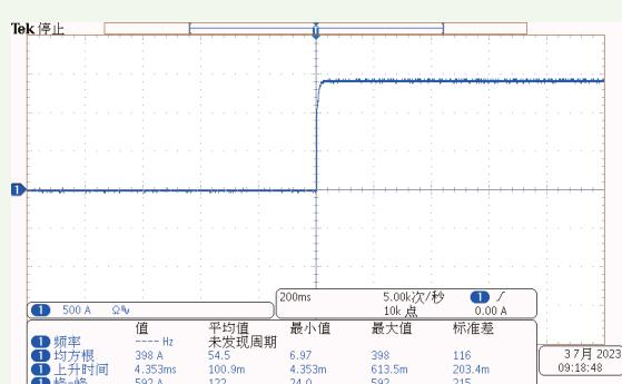
The HY-PMHSU Series is used for practical test of circuit breakers, Current rise time measured  $\leq 10\text{ms}$  (some models)
