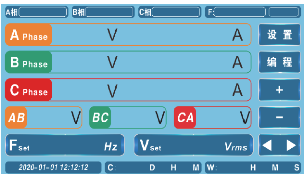
Main interface of three-phase power supply
