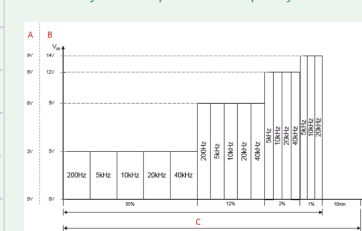
VW 80300 Cycle description with frequency distribution
