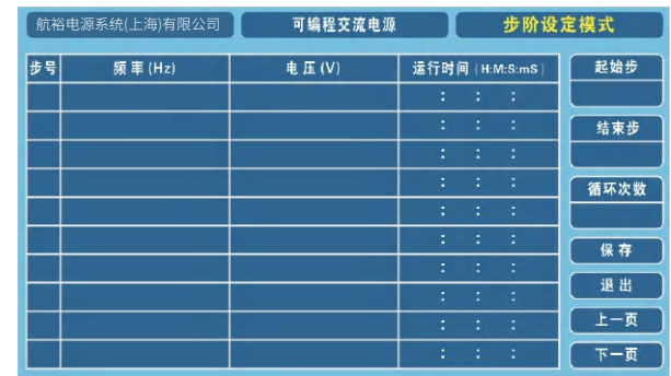
Step setting page can set the required frequency, voltage, Run time, initial step, end step, and number of cycles
