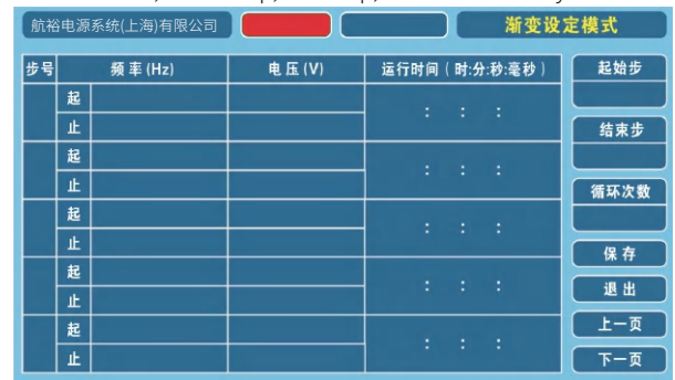
The gradient Settings page can set the required voltage and frequency Run time, initial step, end step
