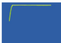
Second-order step response attenuation constant 0.7
