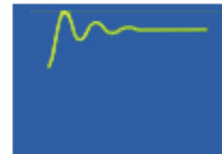
Second-order step response attenuation constant 0.2
