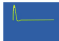
Second-order impulse response attenuation constant 0.7
