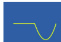
Half wave rectification of sin (negative electrode)
