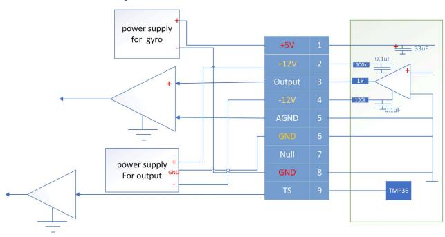
Fig 3 electrical connection
