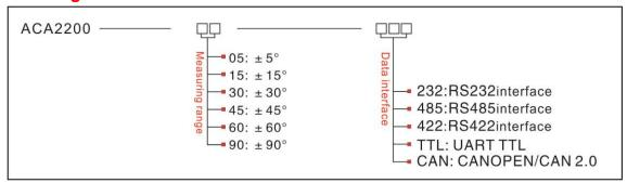
E.g: ACA2200-05-232: Dual-axis/±5°Measuring range/RS232 output
