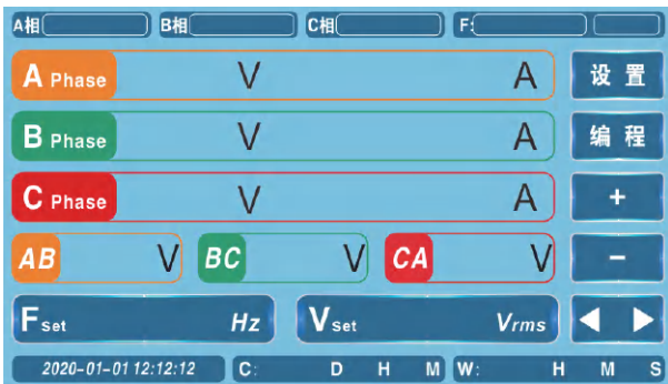
Main interface of three-phase power supply
