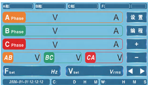
Main interface of three-phase power supply
