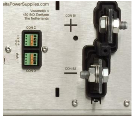
fig 5 - 3 The two DC power terminals CON B1 and B2. Con C and D are the sensing connectors.
