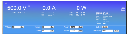
fig 7 - 1 Front console for setting of the output and monitoring various parameters.
