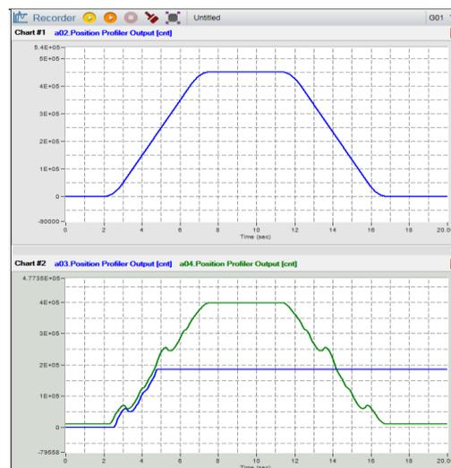
ECAM runs as a single axis function block in the system. Several axes can share the ECAM table. The ECAM runs under the fieldbus DS402 Cyclic/Interpolated position motion modes.
