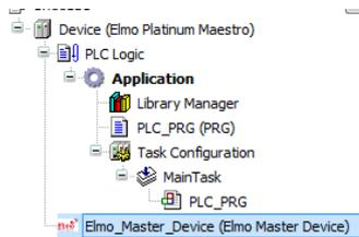
*Scanning For Devices* shall return the Ethercat configuration with the names and Axis References of the Ethercat slaves. Via this configuration – one can map variables to IO's.
