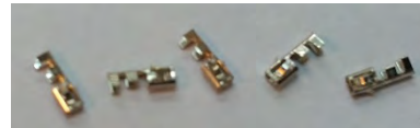
Pins for Single Row Connector MOLEX P/N 501334-0100 Pins for Dual Row Connector MOLEX P/N 501193-3000
