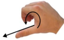
Figure 3-3 Right-hand rule principle two
