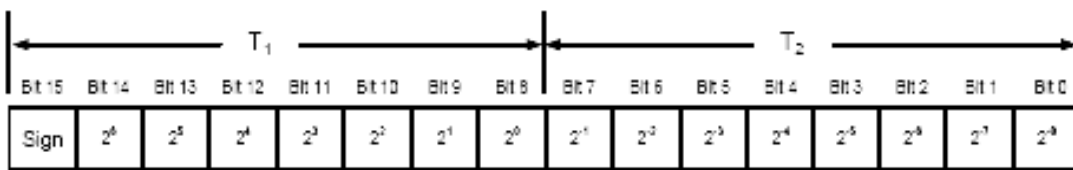
Graph 4 Convert gyro temperature output to [°C]
