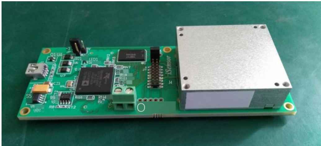
Figure 8. Analog Devices EVAL-ADis Evaluation Board Front Mounted
