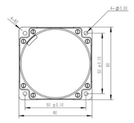
Figure 1 Outline and Installation Diagram of BS-FU35D-1-D1EC Fiber Optic Gyroscope
