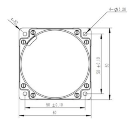
Figure 1 Outline and Installation Diagram of BS-FU35C-1-D1EC Fiber Optic Gyroscope
