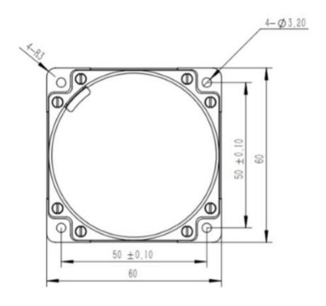
Figure 1 Outline and Installation Diagram of BS-FU35B-1-D1EC Fiber Optic Gyroscope
