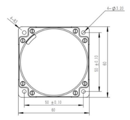
Figure 1 Outline and Installation Diagram of BS-FU35A-5-D1EC Fiber Optic Gyroscope
