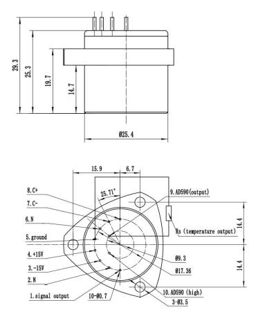
Mark(For temperature selection of version only) :The temperature sensor is AD590,Point 10 is the high power,The point 9 is the low power,The point 9 and power ground use one platinum resistance;The value is 1K,The thermal coefficient is less then 5ppm.
