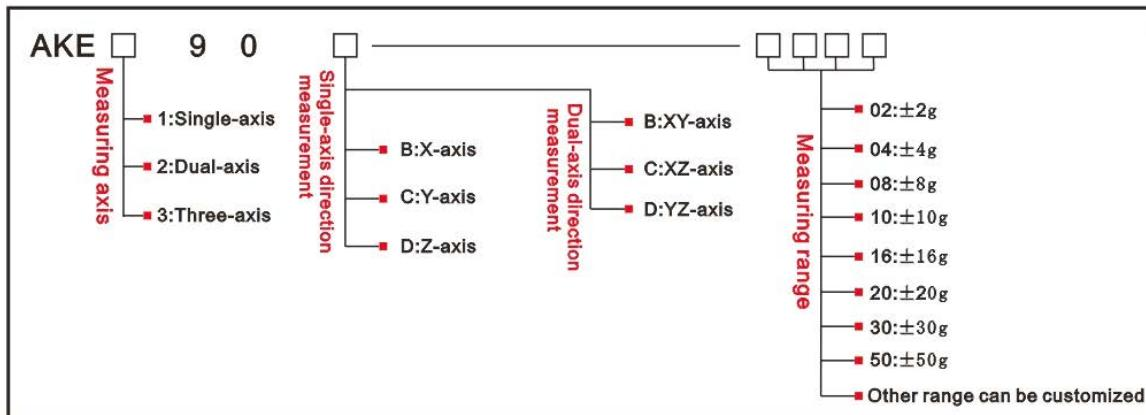
E.g: AKE190B-02: single-axis、X Axis direction measurement、+/-2g selection
