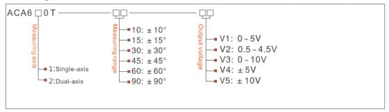
E.g. ACA610T-10-V1: Single-axis/Standard/±10°Measuring range/0-5V Voltage output type **Technical Data**
