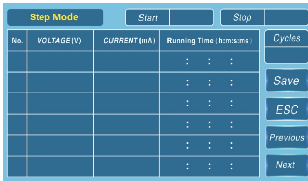
The step setting page can set the required frequency, voltage, running time, initial step, end step and cycle times.
